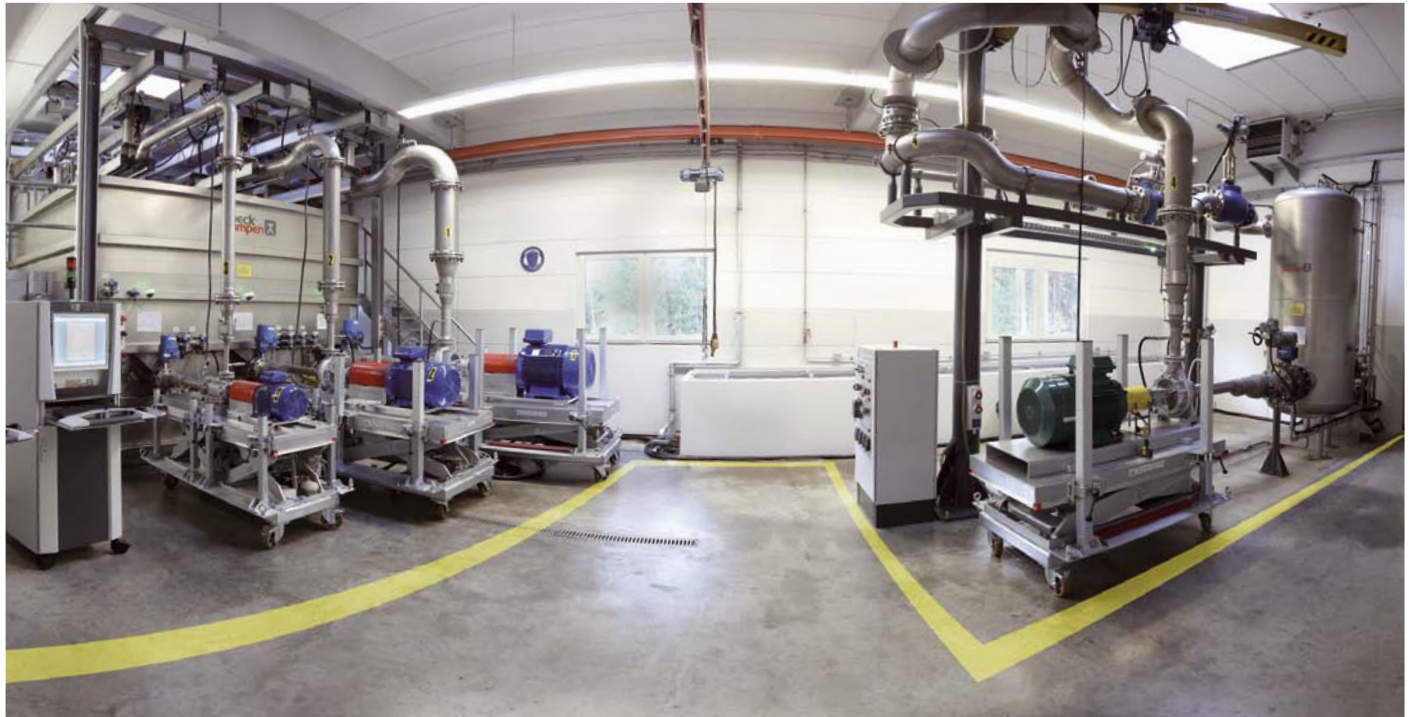
Test stand for liquid pumps on the premises of Speck in Roth Measuring of hydraulics, power requirements, axial thrust, vibrations and NPSH values. Heads of up to 400 m and flow rates of up to 750 m 3 /h.
