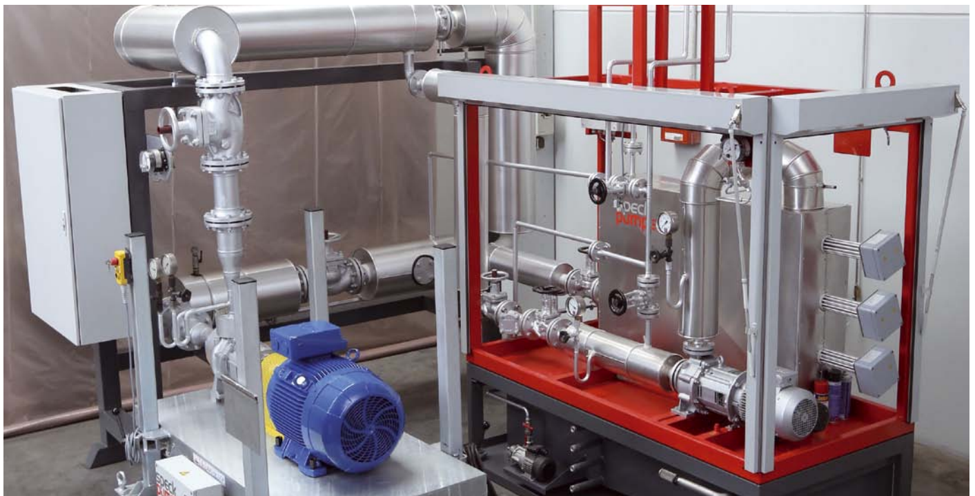
Thermal oil test stand with pump surveillance system on the premises of Speck in Roth. Research of impacts of high temperatures up to 350 °C on the lifetime of the pumps.
