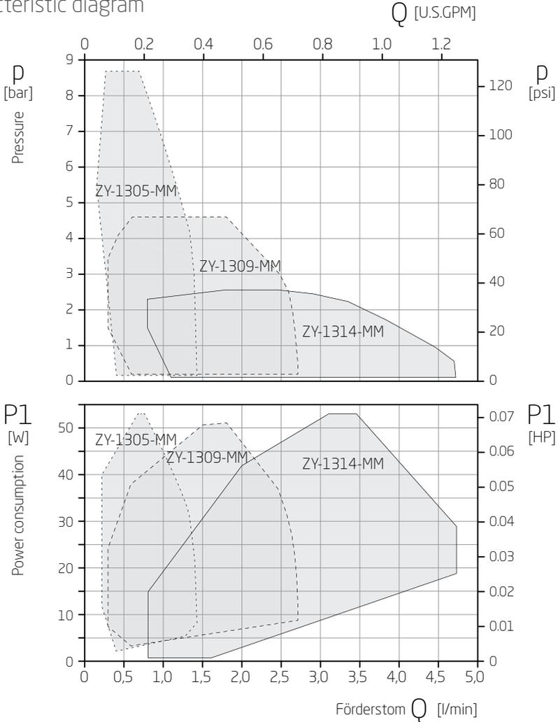
Every operating point can be reached within these characteristic diagrams by setting speed parameters of the drive accordingly.
