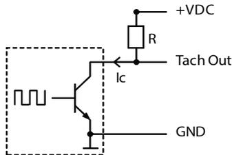
Resistance R has to be selected according to applied voltage VDC, that the current  $I_c$  may not exceed 20 mA. At VDC = 10 V, R usually is approx. 1 k $\Omega$ .
